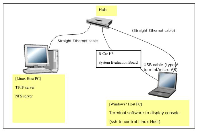
Figure 1 Recommended Environment for R-Car H3 Linux BSP
