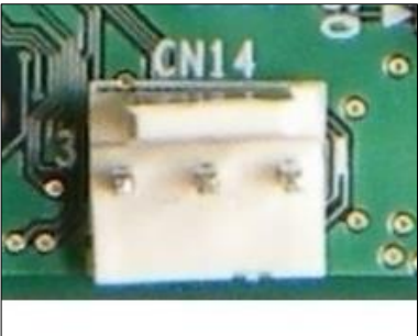
FIGURE 7 FAN CONNECTOR
