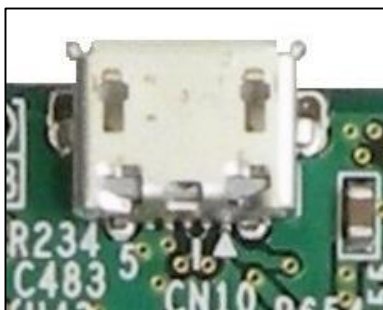
FIGURE 9 DEBUG SERIAL
